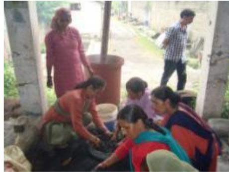
In the Technical Session-IV after the removal of carbonized biomass from the Briquetting Equipments briquettes were prepared by mixing with the clay soil by maintaining proper ratio for better result. Again the pine needles were converted into carbonized biomass in all the Equipments by the participants and kept for cooling at the venue.
